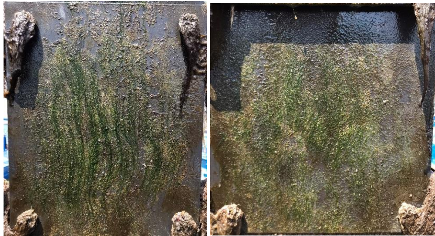
Figure 6: Algae growth on Jotun A (left) and B (right) during the first inspection date (T1). Note that macroalgae coverage is calculated using only the initial attachment points.
