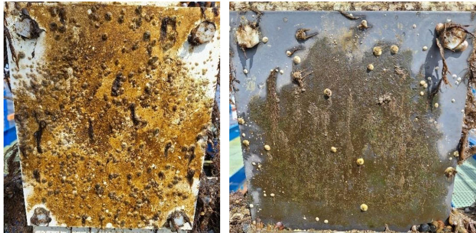
Figure 11: Left: Nautix B T2 with barnacle growth. Algae was attached to the barnacles but not to the panel. Right: Trilux A T2 with barnacle growth and hydroids.
