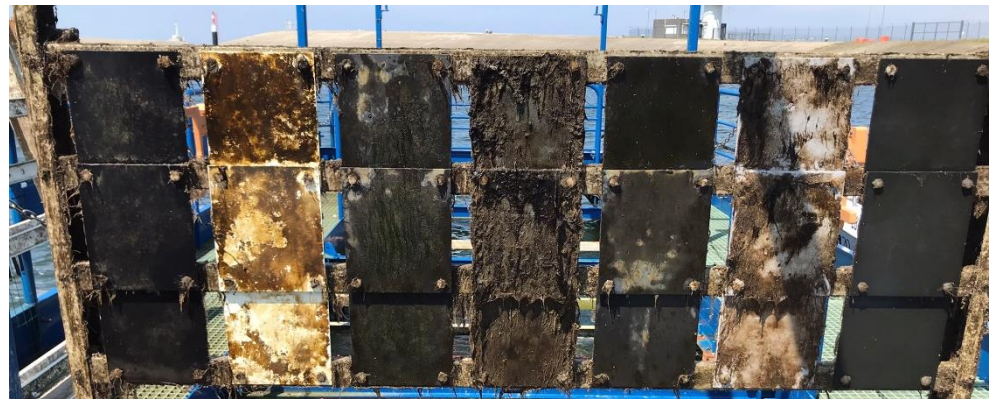
Figure 4: Biofouling growth on coated panels after 5 weeks of exposure (T1) – from left to right: Hempablue, Nautix, Jotun, PVC (control), Trilux, Intersleek and Hempaguard. Three replicas of each coating are stacked vertically and denoted as A, B, and C from top to bottom.
