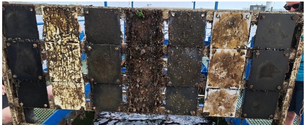
Figure 12: Biofouling growth on coated panels after 15 weeks of exposure (T3) – from left to right: Hempablue, Nautix, Jotun, PVC (control), Trilux, Intersleek and Hempaguard. Three replicas of each coating are stacked vertically and denoted as A, B, and C from top to bottom.
