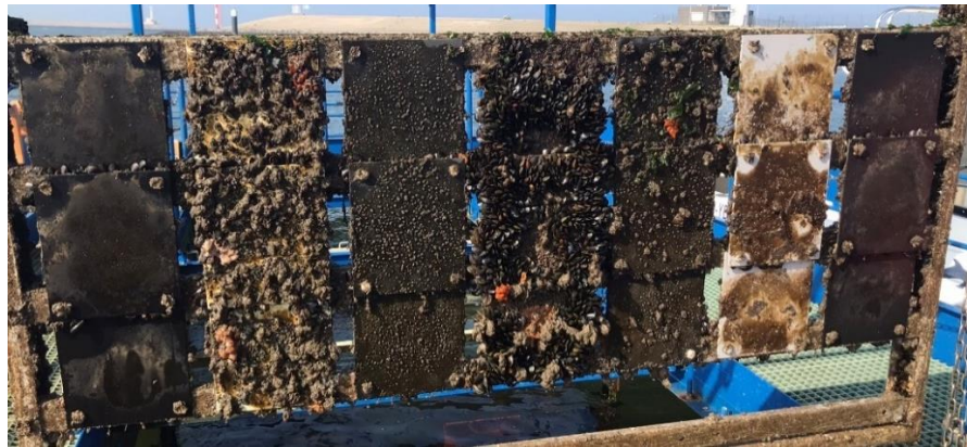
Figure 15: Biofouling growth on coated panels after 20 weeks of exposure (T4) – from left to right: Hempablue, Nautix, Jotun, PVC (control), Trilux, Intersleek and Hempaguard. Three replicas of each coating are stacked vertically and denoted as A, B, and C from top to bottom.
