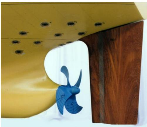
The signals from the pressure transducers are sampled and digitised. In order to remove the influence of small changes in the propeller rotation rate, the measurements are resampled to 360 samples per revolution, based on the measured blade angular position. These resampled signals are equidistant with respect to blade position, but not necessarily with respect to time. In order to ensure that the blade passage frequency (BPF) is well captured, only complete revolutions are considered.
